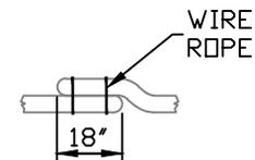
FOR FILTER SOCK, OVERLAP JOINT BY 18" AND SECURE WITH 2 WIRE ROPES
