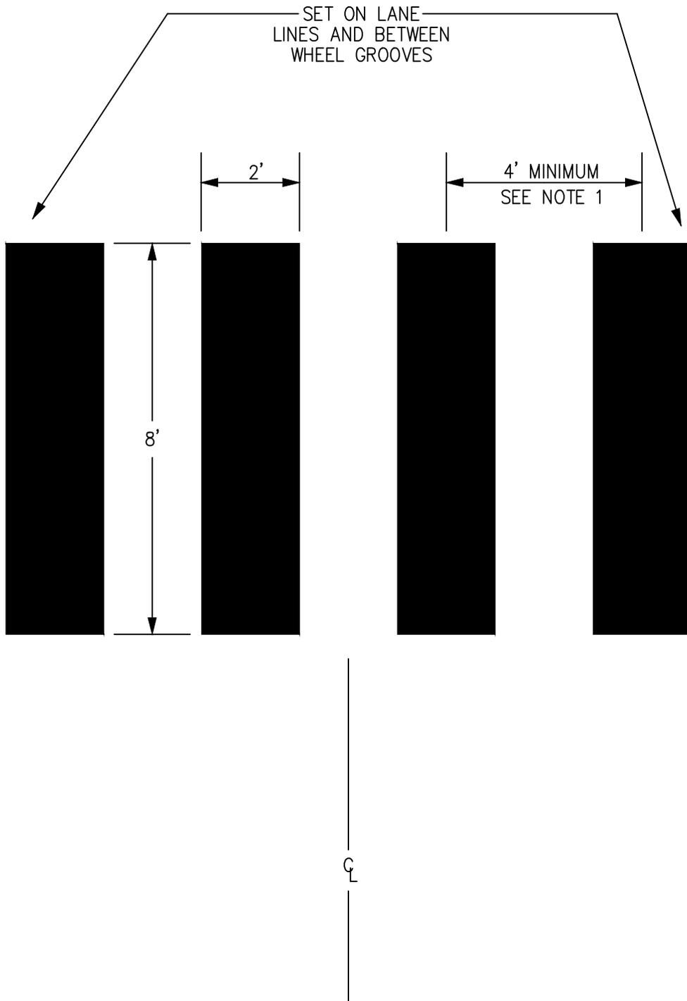
FIELD ADJUST SPACING TO AVOID VEHICLE TIRE PATHS.
