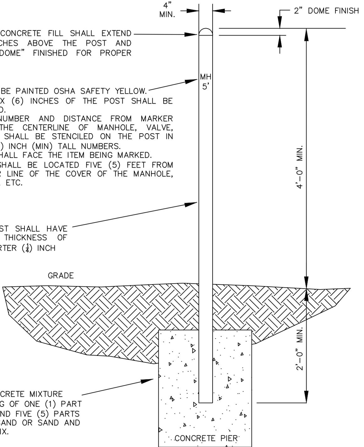
NOTE: PIPE SHALL BE BLASTED (OR OTHERWISE CLEANED) PRIOR TO PRIMING AND PAINTING. THE PIPE SHALL BE COATED WITH TWO (2) LAYERS OF PRIME COAT AND ONE (1) OIL BASE SEMI-GLOSS FINISHING COAT IN THE COLORS SPECIFIED ABOVE. THE TOTAL PRIME AND PAINT THICKNESS SHALL BE A MIN. OF 4.5 MIL. THICKNESS OR 1.5 MIL. OF EACH LAYER.
