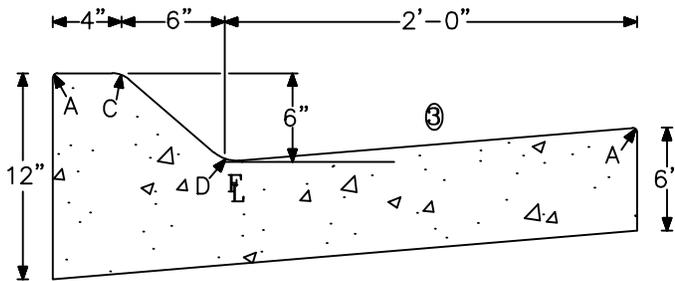
TYPE 2 CURB & GUTTER (SECTION IIM)
