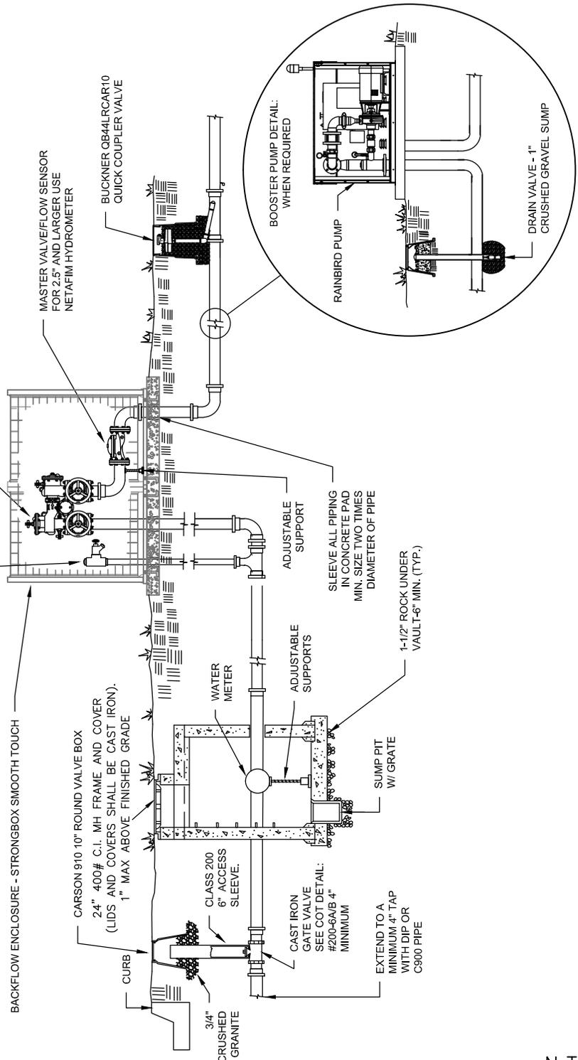
RAIN SHUT-OFF DETAIL WITH POLE ASSEMBLY
