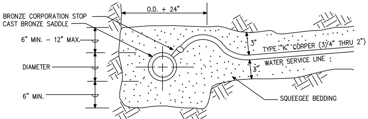
NOTE: BEDDING MATERIAL SHALL BE SQUEEGEE NON-FRACTURED ROUNDED AND SHALL CONFORM TO THE FOLLOWING LIMITS WHEN TESTED BY MEANS OF LABORATORY SIEVES:
