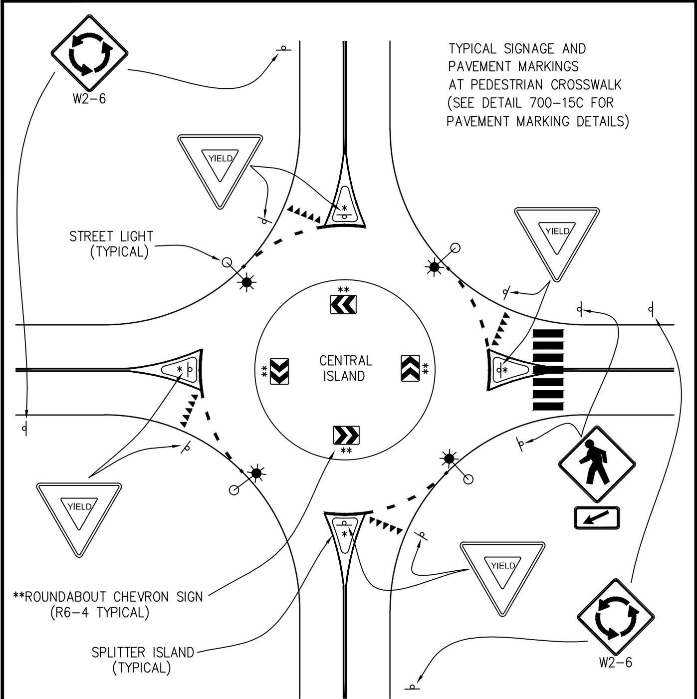
TYPICAL SIGNAGE AND PAVEMENT MARKINGS AT PEDESTRIAN CROSSWALK (SEE DETAIL 700-15C FOR PAVEMENT MARKING DETAILS)
