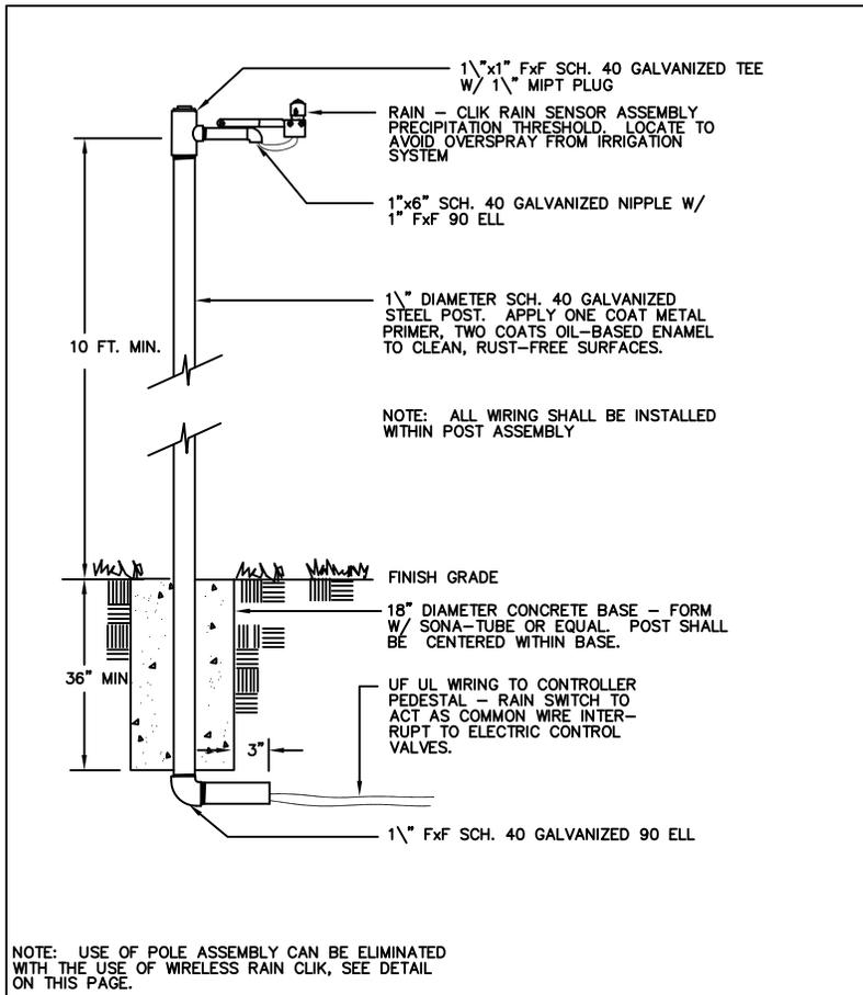
WIRELESS RAIN SHUT-OFF DETAIL
