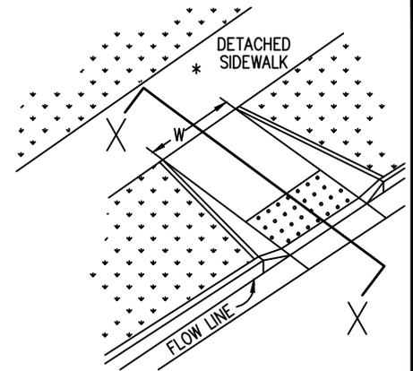
\* SLOPE MUST BE < 2.0% IN BOTH DIRECTIONS
