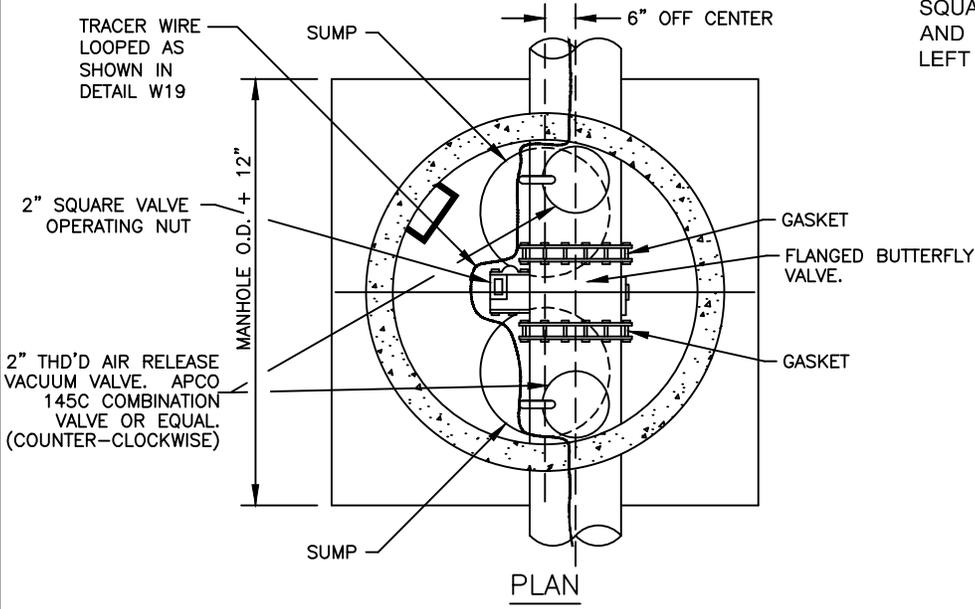
NOTE: BUTTERFLY VALVES SHALL BE CLASS 150-B AND CONFORM TO AWWA SPECIFICATION C-504
