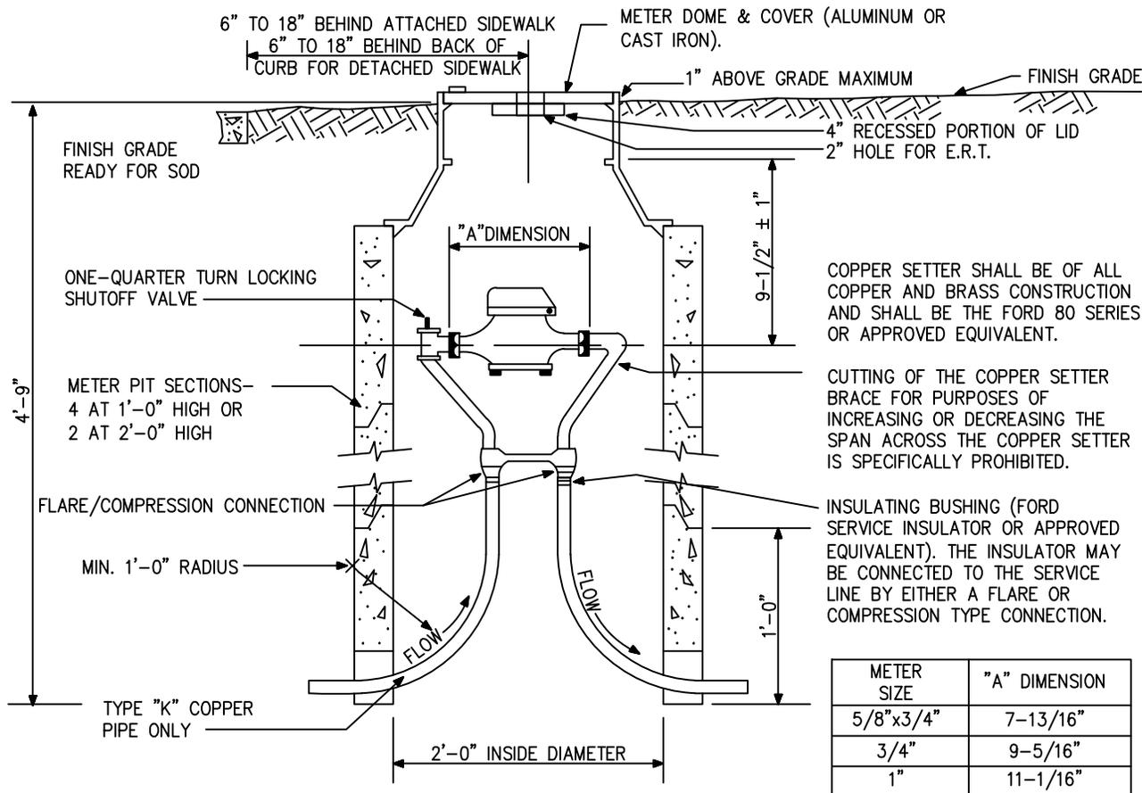
IF SERVICE LINE IS A DIFFERENT SIZE THAN THE METER, THEN THE REDUCTION SHALL OCCUR OUTSIDE THE METER PIT.
