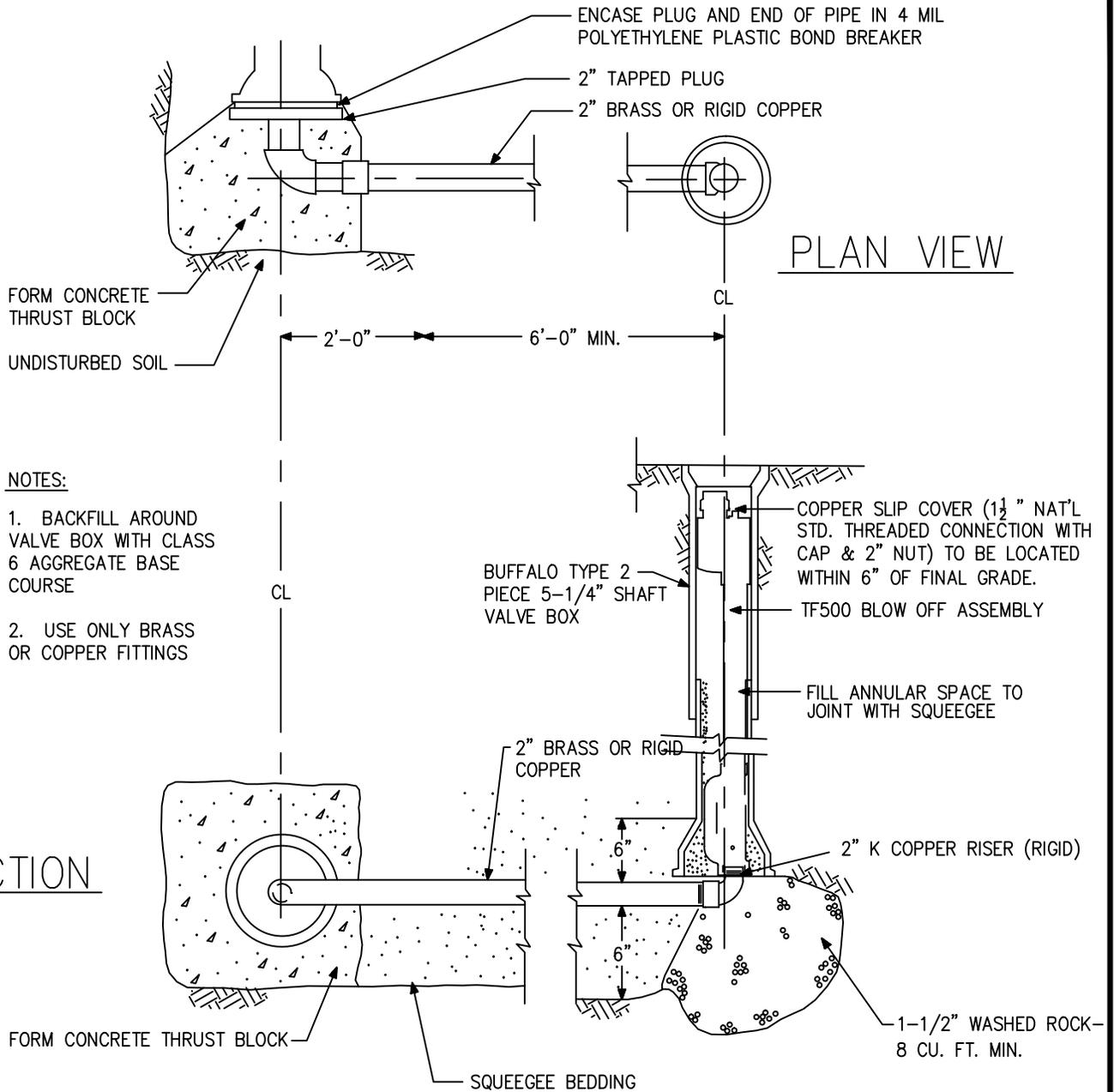
VALVES SHALL BE HANDLED IN SUCH A MANNER AS TO PREVENT ANY INJURY OR DAMAGE AND SHALL BE THOROUGHLY CLEANED BEFORE INSTALLATION. VALVES SHALL BE SET IN SUCH A MANNER THAT THE VALVE STEMS ARE PLUMB. VALVE BOXES SHALL BE INSTALLED PLUMB. FINAL ELEVATION OF THE VALVE BOXES SHALL BE LEFT TO THE DISCRETION OF THE DEVELOPMENT ENGINEERING MANAGER.
