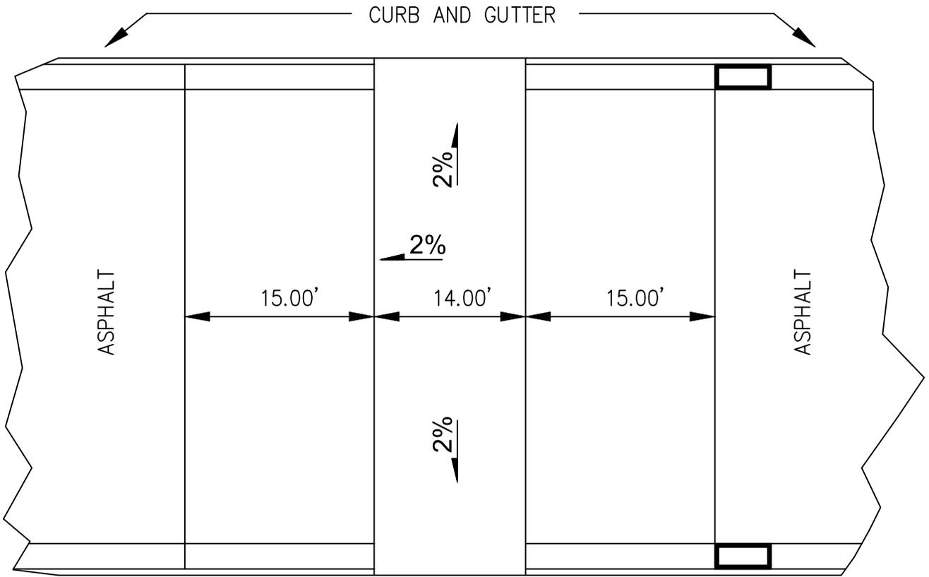
STORM INLETS REQUIRED AT HIGH POINT OF APPROACH TO SPEED TABLE
