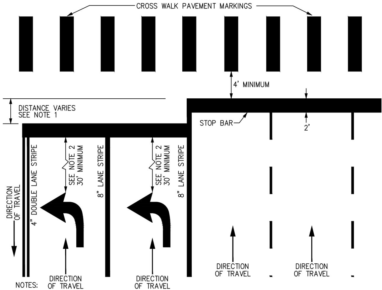
1. DISTANCE TO BE FIELD DETERMINED TO ACCOMMODATE TURNING RADIUS; LAYOUT TO BE APPROVED BY THE TRAFFIC ENGINEER PRIOR TO INSTALLATION.
