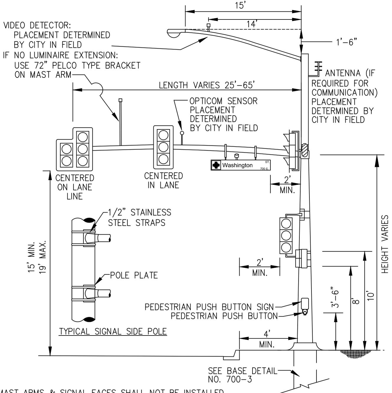
MAST ARMS & SIGNAL FACES SHALL NOT BE INSTALLED UNTIL FIVE (5) DAYS OR LESS PRIOR TO ACTIVATION UNLESS APPROVED BY THE TRAFFIC ENGINEER.
