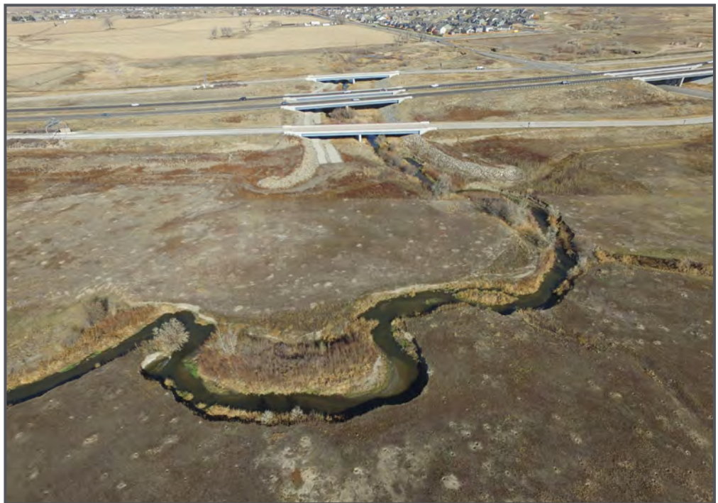
Aerial view of the pilot project site looking north towards E-470; Big Dry Creek is migrating laterally and causing heavy bank erosion due to the straightening of the channel on both the north and south sides of the site
