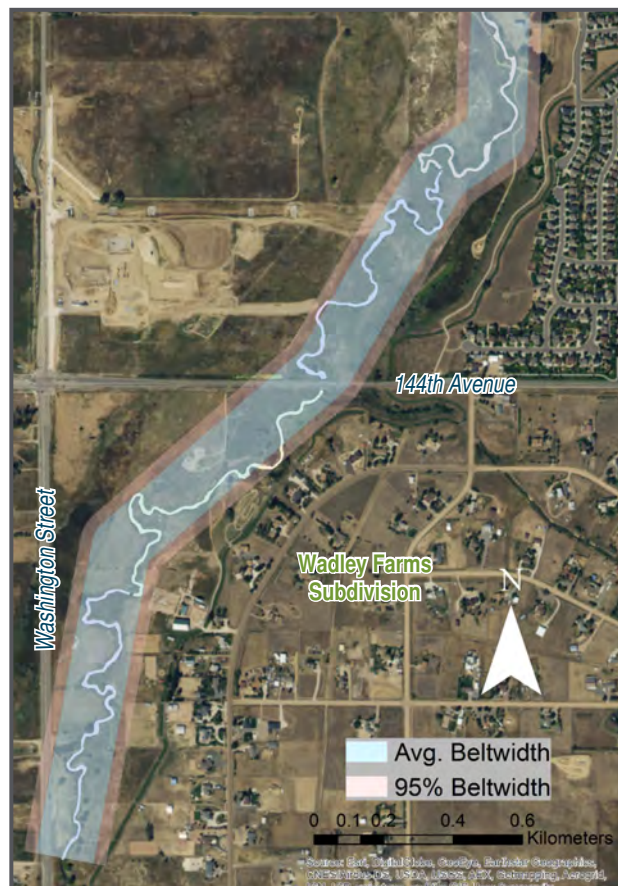
Estimated Average and 95th Percentile Meander Belt width for Big Dry Creek through the southern project area
