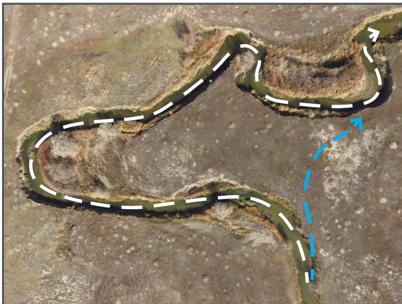
If the channel's meander is straightened out, the water will be falling the same height over a shortened length, increasing the creek's slope and resulting in the need for grade control structures
