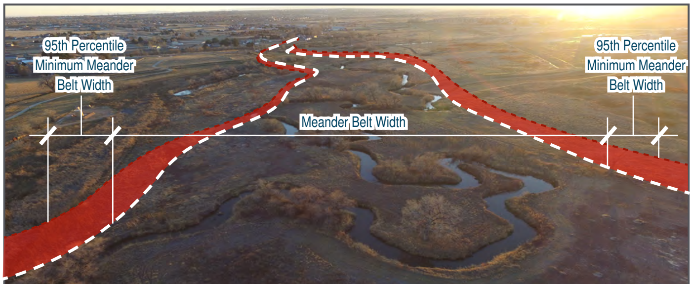
The meander belt identifies an area adjacent to the stream, where land is subject to erosion by the stream channel; this meander belt width is overlaid on an aerial of Parcel III
