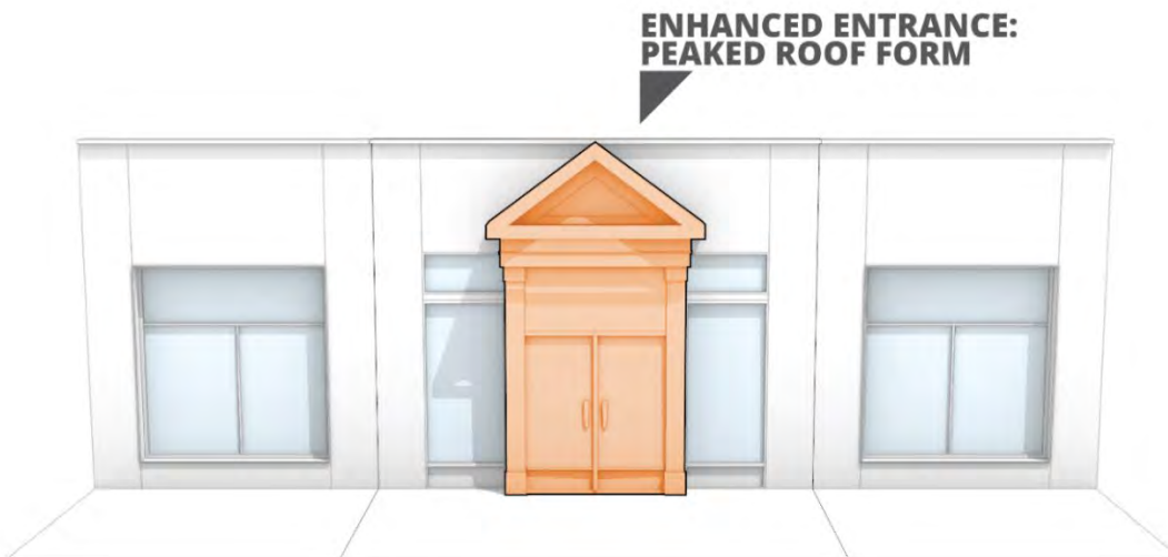
Figure 18-550.3. Example of a peaked roof form.
