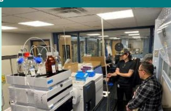
Thornton's water treatment lab has a Liquid Chromatography-Mass Spectrometry (LCMS) instrument that detects and measures tiny amounts of per- and polyfluoroalkyl substances (PFAS) in water samples.
