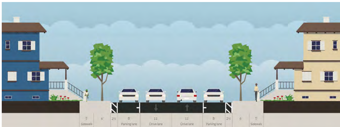
Figure 5.13 Example Local Street Cross Section
