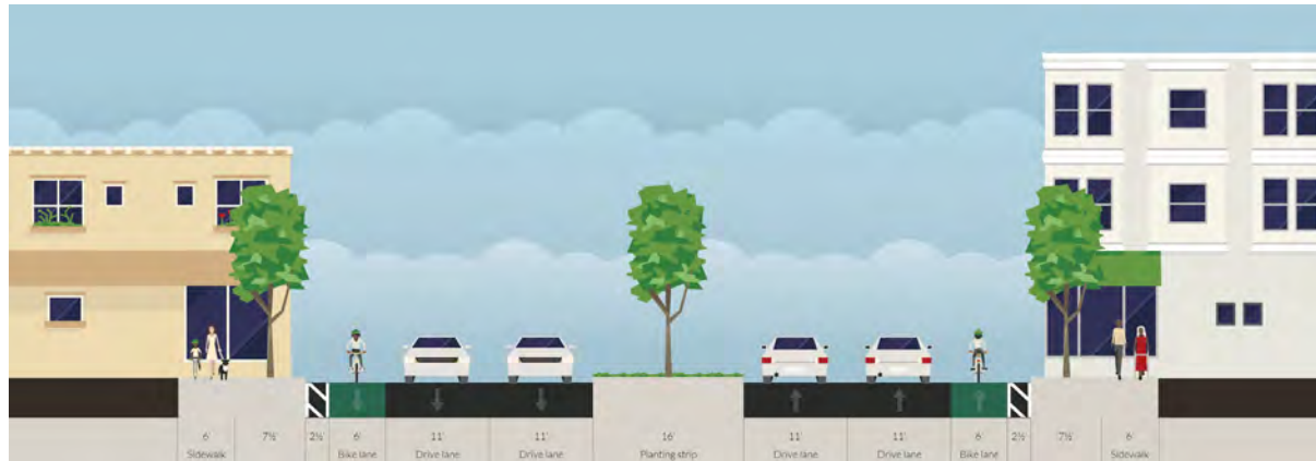
Figure 5.10: Cross Section of Welby Road North of Transit Station
