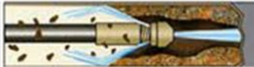
Acceptable: Hydrojet clears blockage
