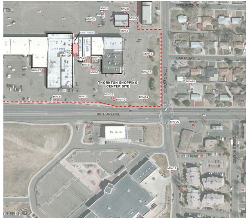
A former dry cleaner in the Thornton Shopping Center released chemicals, namely PCE, that need to be monitored. The red circles show the locations of groundwater monitoring wells installed in the community to monitor the groundwater. Drinking water is not affected.
